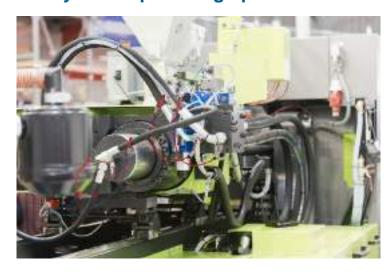
**MB SAFEBLOCK** is a special safety system for high pressure flexible hoses, expressely designed to arrest the movement of the hose in case of disconnection of the fittings, preventing serious damages to person and machineries in the vicinity.
