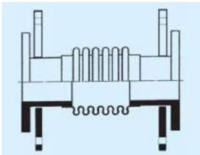
**EXPANFLEX MB-E1** is an axial Type Approved multiwall expansion joint, without circumferential weld. Made in AISI 321 Stainless Steel T.I.G. welded, or with other grades of Stainless Steel upon request.
