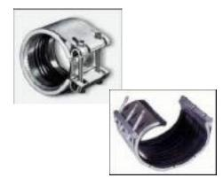
Built in a simple way, it is the most technically advanced, practical and economical instrument for the maintenance responsible for both naval and insutrial installations. They can be be used in the presence of axial movements. The toothed conical ring perfectly adheres to the surface of the pipe, giving the joint an excellent resistance to vibration and, thanks to special internal seals, is ensured a perfect seal.
