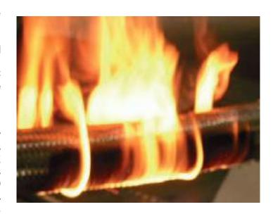
Stainless Steel AISI 304 external reinforcement to provide higher mechanical resistance.
