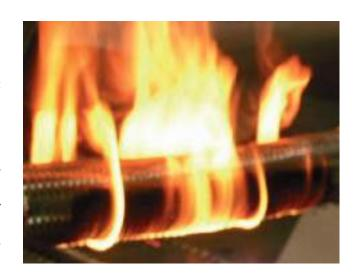
To satisfy the above mentioned requirements, **MB LUBE OIL GOLD 29** has been tested by applying a flame for 30 minutes at the required temperature of 800 +/- 50°C with a working pressure of 5 bar. The specimen is than tested at a pressure twice the working parameter for 15 minutes, in order to confirm that the flexible hose is in conformity with the specifications.
