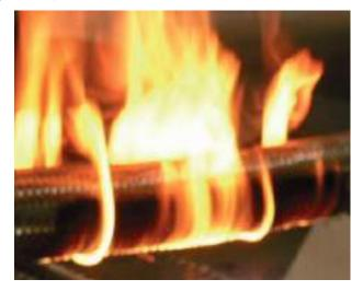
To satisfy the above mentioned requirements, **MB HFO FUEL OIL PLUS** has been tested by applying a flame for 30 minutes at the required temperature of 800 +/- 50°C with a working pressure of 5 bar. The specimen is than tested at a pressure twice the working parameter for 15 minutes, in order to confirm that the flexible hose is in conformity with the specifications.
