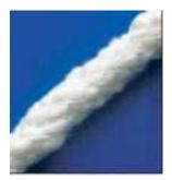
**C3V** glass insulating rope consists of glass fibres, without any binding agents, enclosed in a open nesh knit braided sleeving. This product is mainly used for insulating piping.
