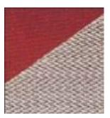
Fiberglass fabric "E type ", one side coated with red silicone rubber.
