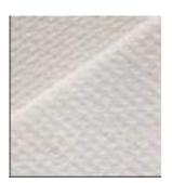
Glass cloth woven from textured "E" glass fibres and coated on both sides with white silicone rubber.
