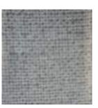
Made with P.A.N (polyacrylonitrile) yarn fibers and synthetic fibers characterized by high mechanical resi stance. Very good properties in thermal insulation, nonflammable. It does not melt. Coated one side with uncured natural rubber.
