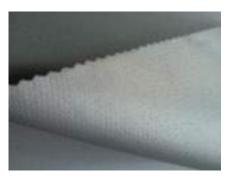
Fiberglass fabric "E type", each side coated with grey silicone rubber.
