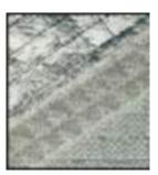
Fabric fibers made of "E" glass continuous filament, double-gridded texture. Aluminized version also available.
