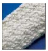
Texturized glass fiber sleeve, silicon coated version also available for waterproof applications at temperatures not exceeding 200 °C.
